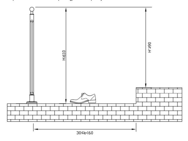
The distance b between the railing from the last stair stone should satisfy 30 cm≤b≤60 cm. In this way even if a person stumbles upon the stair stone, the risk of an accident is minimized.
