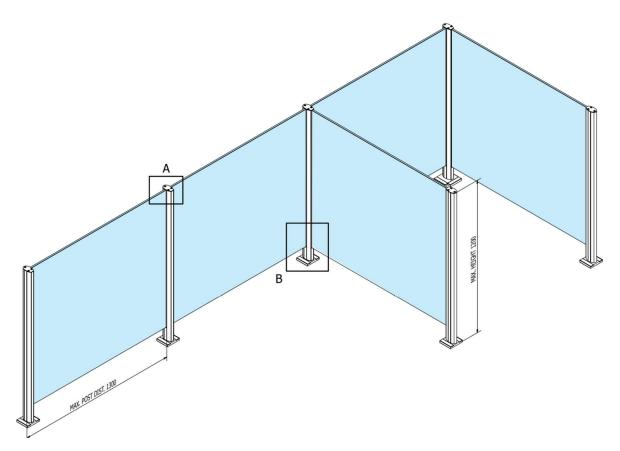
Maximum height 1.20 m and width 1.30 m for typical railing applications.
