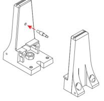
Adjustable feet from above for the levelling of the railing;
